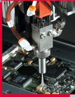
The PVA650 is the platform of choice for economical, flexible adhesive and coating process solutions. Configurable for virtually any adhesive application, the PVA650 is ideal for most selective conformal coating, potting, dot, and bead operations. Multiple applications can be implemented on one gantry platform for a higher ROI (return on investment) and greater capability in your manufacturing process.
