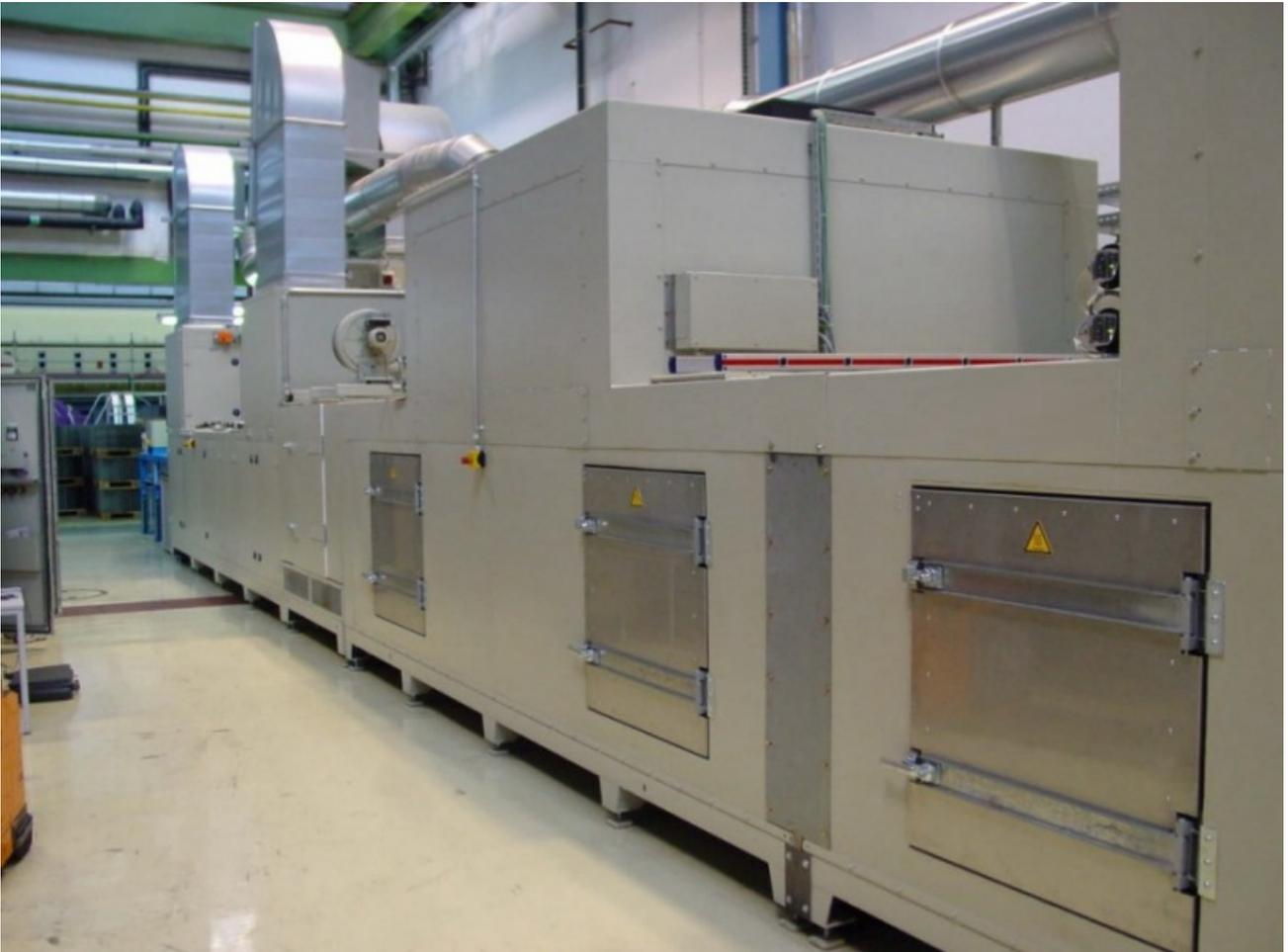
KNÖDEL segment coating line, coating dryer and cooling section
